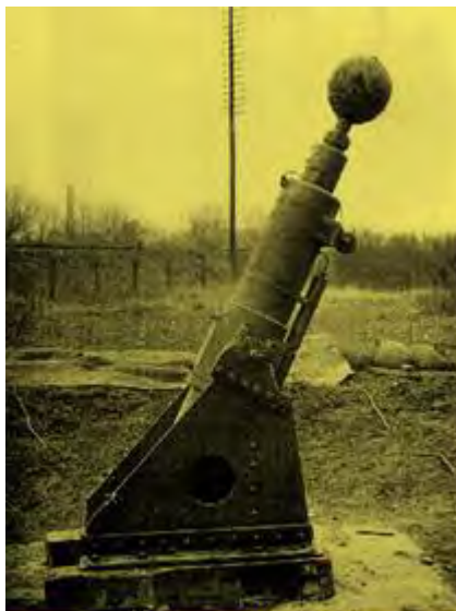
Constantinescu' s sonic gun ; the spherical bullet is external, mounted at the muzzle LS Cozna
